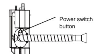
3.After used up disinfectant liquid, put some water in the tank and work around 1-2 minutes to avoid the disinfectant liquid blocking or corroding the nozzles and pipes.
